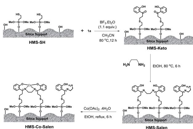
**Figure 2.** Schematic diagram of the procedure to immobilize salen-type cobalt(II) schiff base complex.
