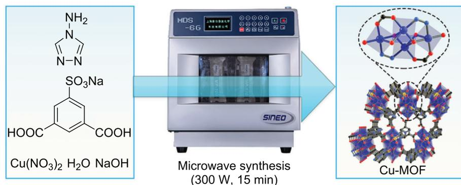
**Scheme 1** Microwave-assisted synthesis of  $[\text{Cu}_4(\mu_3\text{-OH})_2]$ -cluster-based metal-organic framework (Cu-MOF)
