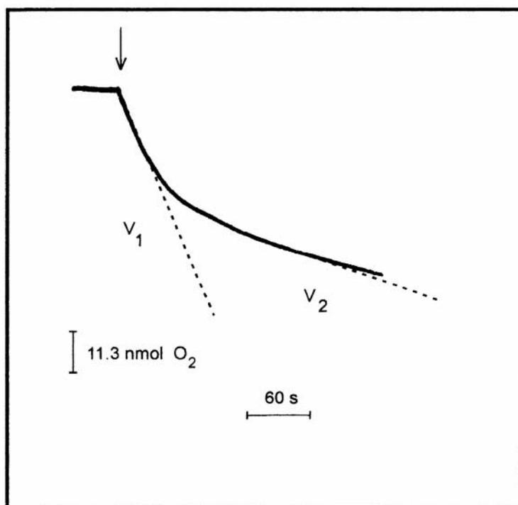
Fig. 1. Typical record of NADPH (1 mM)-initiated oxygen uptake by the buffered (pH 7.7, 40 mM Tris-HCl) reaction mixture (1 cm<sup>3</sup>) containing 1 mM Na<sub>2</sub>EDTA, 1 mM MgCl<sub>2</sub>, 0.6 μM FNR and 20 μM duroquinone (or other quinones). V<sub>1</sub>, rate of oxygen uptake during the 1st minute of measurement; V<sub>2</sub>, rate of oxygen uptake between 2nd and 3rd minutes of measurement.
