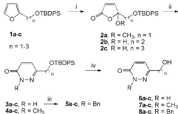
**Scheme 1.** Reagents and conditions: (i) (1) O<sub>2</sub>, *hν*, rose Bengal, MeOH,  $-78^\circ\text{C}$ , (2) Ac<sub>2</sub>O, Py, DMAP, rt for **2a**; or O<sub>2</sub>, *hν*, rose Bengal, DIPEA, MeOH,  $-78^\circ\text{C}$  for **2b–c**; (ii) NH<sub>2</sub>NH<sub>2</sub>·H<sub>2</sub>O or CH<sub>3</sub>NHNH<sub>2</sub>, EtOH, reflux or  $0^\circ\text{C}$ ; (iii) NaH, BnBr, Bu<sub>4</sub>NI, THF, rt; (iv) TBAF, THF, rt.
