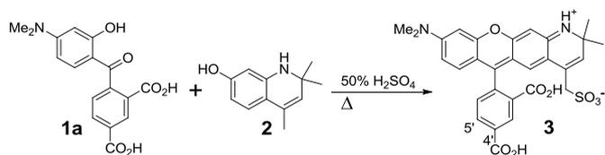
**Scheme 3.** Condensation of benzophenone **1a** with aminophenol **2**. (**1a** + 1.2 eq. **2**, 50% H<sub>2</sub>SO<sub>4</sub>, 125 °C, 2 hr, reverse phase HPLC purification, Yield **3** 10.4%)
