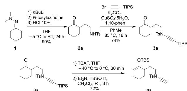
**Scheme 1.** Synthesis of the silyl enol ether **4a**. TBAF = tetra-*n*-butylammonium fluoride, TBS = *tert*-butyldimethylsilyl, Tf = trifluoromethanesulfonyl, THF = tetrahydrofuran, TIPS = triisopropylsilyl, Ts = 4-toluenesulfonyl.
