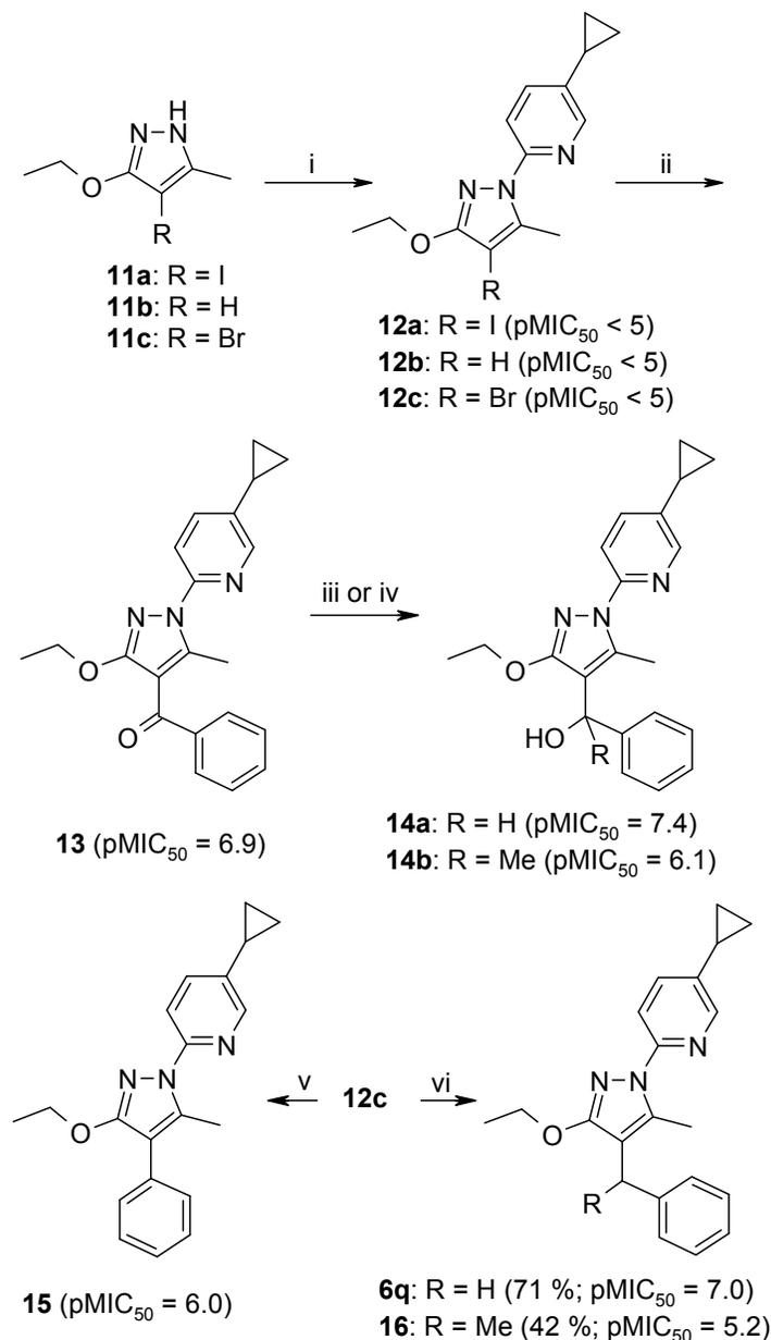
Scheme 1. 5-cyclopropyl-2-fluoropyridine (**5q**), MeCN, microwave 180 °C 12h. ii: a) BuLi, THF, -78 °C, b) PhCOCl, -78  $\rightarrow$  20 °C. iii: NaBH<sub>4</sub>, EtOH. iv: MeLi; THF, 20 °C. v:
