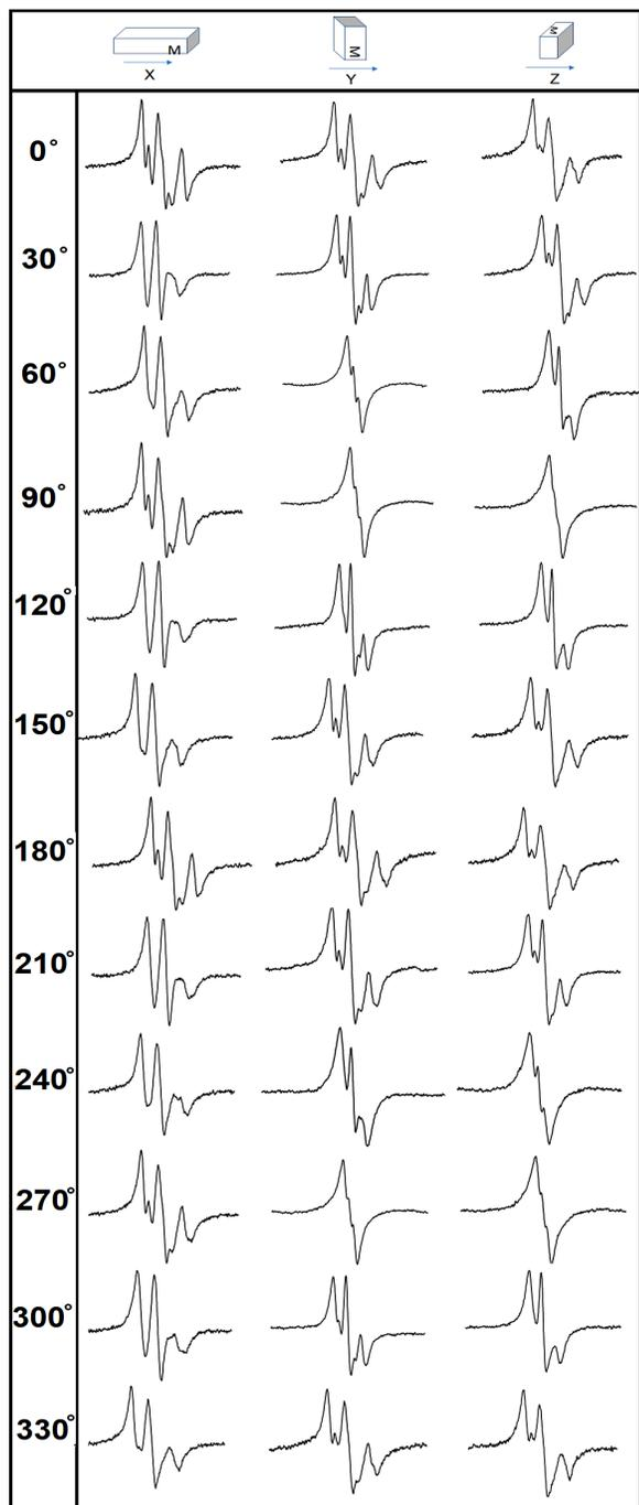
**Figure 5.** Single-crystal EPR measurements of a 1:1 diluted crystal of UCLA-NO analyzing each orientation of the crystal from 0° to 330° in 30° increments.
