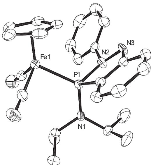
**Fig. 5.** ORTEP diagram showing the structure of **10**. Thermal ellipsoids are shown at the 50% level. Hydrogen atoms and the  $\text{AlCl}_4^-$  counterion have been omitted. Selected distances (Å) and angles (deg): Fe–P = 2.2347(9), P–N1 = 1.652(2), P–N2 = 1.716(2), P–C14 = 1.796(3), N2–N3 = 1.428(3), N3–C15 = 1.412(4), C14–C15 = 1.375(4), N1–P–C14 = 112.2(1), N2–P–C14 = 89.9(1), N3–N2–P = 113.6(2), C15–N3–N2 = 109.4(2), C15–C14–P = 110.6(2), C14–C15–N3 = 115.1(3).
