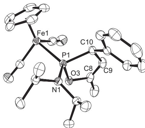
**Fig. 4.** ORTEP diagram showing the structure of **8**. Thermal ellipsoids are shown at the 50% level. Hydrogen atoms and the  $\text{AlCl}_4^-$  counterion have been omitted. Selected distances (Å) and angles (deg): Fe–P = 2.2129(5), P–N = 1.643(1), P–O3 = 1.650(1), P–C10 = 1.883(1), O3–C8 = 1.400(2), C10–C9 = 1.505(2), C9–C8 = 1.320(3), C10–P–O3 = 94.41(7), P–O3–C8 = 112.3(1), O3–C8–C9 = 116.1(1), C8–C9–C10 = 116.1(2), C9–C10–P = 101.1(1).
