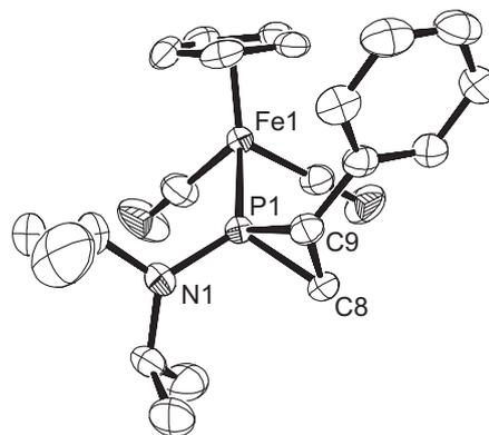
Fig. 2. ORTEP diagram showing the structure of [CpFe(CO)<sub>2</sub>{P(N-*i*-Pr<sub>2</sub>)CH(Ph)CH<sub>2</sub>}] [AlCl<sub>4</sub>] (**4a**). Thermal ellipsoids are shown at the 50% level. Hydrogen atoms and the AlCl<sub>4</sub><sup>-</sup> counterion have been omitted. Selected distances (Å) and angles (deg): Fe–P = 2.2272(6), P–N = 1.649(2), P–C8 = 1.800(2), P–C9 = 1.850(2), C9–P–C8 = 49.3(1), P–C9–C8 = 67.1(1), P–C8–C9 = 63.7(1).
