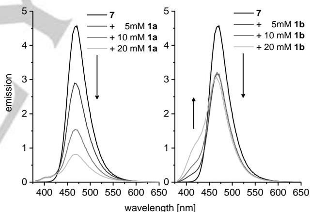
**Figure 2.** Fluorescence quenching of **7** (2  $\mu$ M) by substrates **1a** (left) and **1b** (right) in MeCN. Excitation  $\lambda_{exc}$ =365 nm.
