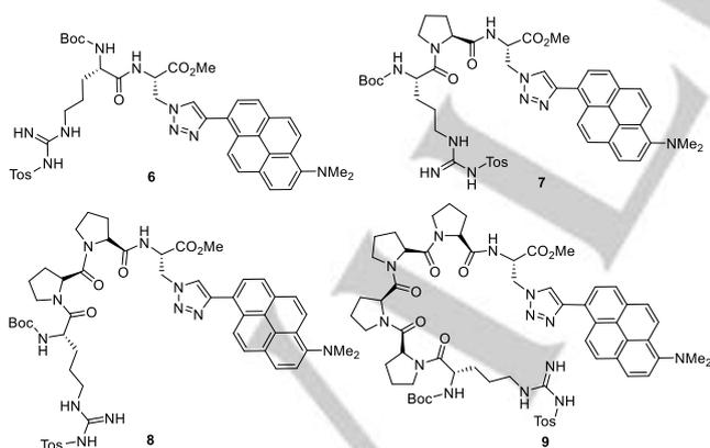
**Scheme 2.** Photocatalytic peptides **6-9** with the **Py** chromophore as side chain in an Ala derivative. The schematic drawings show only the chemical constitution and configuration of the peptides and should not imply a precise conformation.
