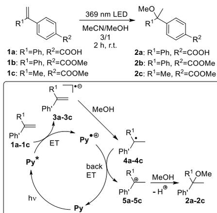
**Scheme 1.** Photocatalytic Markovnikov-type nucleophilic addition of MeOH to substrates **1a-1c** and proposed photocatalytic mechanism for the conversion to products **2a-2c** using **Py**-containing peptides as photoredox catalysts.
