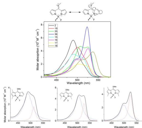
**Figure 3.** Main resonance structures resulting from the electronic coupling of the 8-methylthio group with the BODIPY core and absorption spectra of dye **2** and its non-symmetric (**15-19**) and symmetric (**35-36**) alkylated derivatives. For the sake of clarity, the absorption band of selected representative compounds (**15**, **35** and **16**) has been deconvoluted in two Lorentzians.
