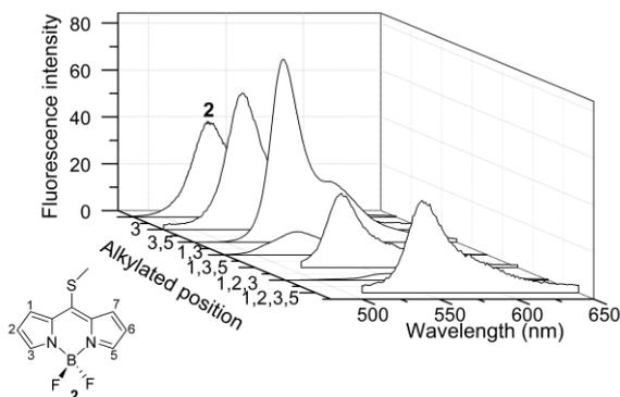
**Figure 4.** Evolution of the fluorescence spectra with regard to the alkylated chromophoric position of the BODIPYs bearing the 8-methylthio group (compound **2**).
