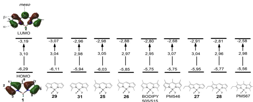
**Figure 1.** HOMO and LUMO energies (eV) of alkyl-BODIPYs. The corresponding contour maps of the simplest compound **1** are included for a better rationalization of the alkylation effect.
