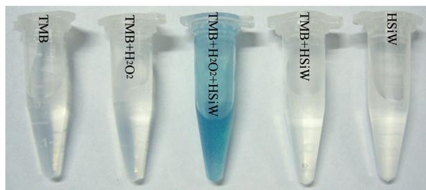
**Figure 1.** Photographs of solutions of TMB, TMB + H<sub>2</sub>O<sub>2</sub>, TMB + HSiW + H<sub>2</sub>O<sub>2</sub>, TMB + HSiW, and HSiW in pH 4.0 NaAc buffer ([TMB] = 0.1 mM, [H<sub>2</sub>O<sub>2</sub>] = 44 mM, [HSiW, H<sub>4</sub>SiW<sub>12</sub>O<sub>40</sub>] = 1.5 mM).
