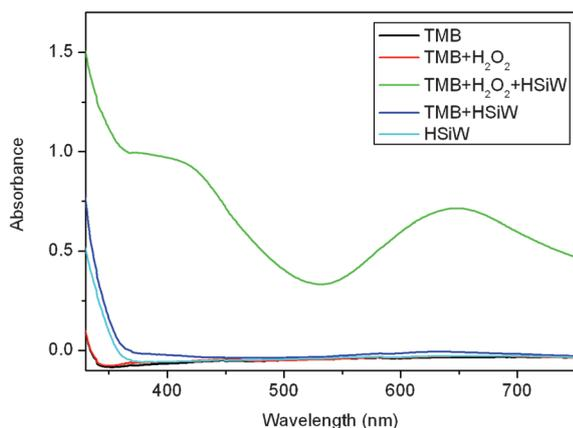
**Figure 2.** UV/Vis spectra of solutions of TMB, TMB + H<sub>2</sub>O<sub>2</sub>, TMB + HSiW + H<sub>2</sub>O<sub>2</sub>, TMB + HSiW, and HSiW in pH 4.0 NaAc buffer ([TMB] = 0.1 mM, [H<sub>2</sub>O<sub>2</sub>] = 44 mM, [HSiW, H<sub>4</sub>SiW<sub>12</sub>O<sub>40</sub>] = 1.5 mM).
