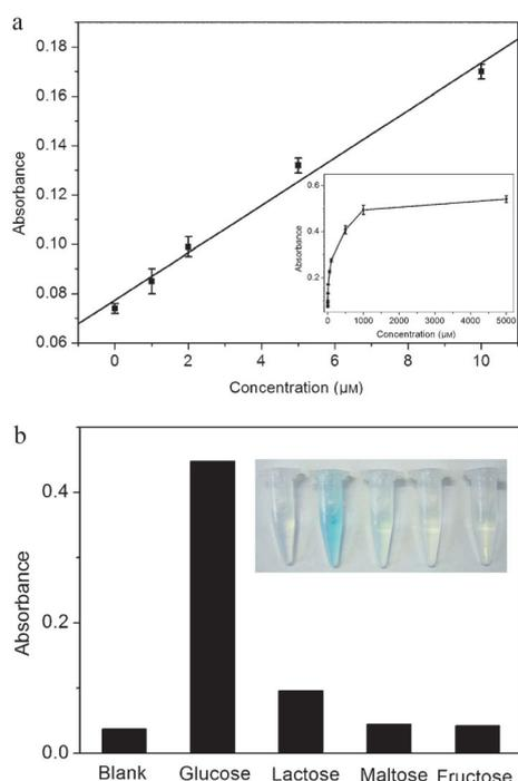
**Figure 4.** a) The linear calibration plot of the absorbance at 651 nm on the concentration of glucose from 0 to 10  $\mu\text{M}$ . The inset shows dependence of the absorbance at 651 nm on the concentration of glucose in the range from 0 to 5 mM. b) Determination of the specificity of GOx for glucose detection with 5 mM lactose, 5 mM maltose, 5 mM fructose, and 1 mM glucose. The inset shows color change with the different solutions.
