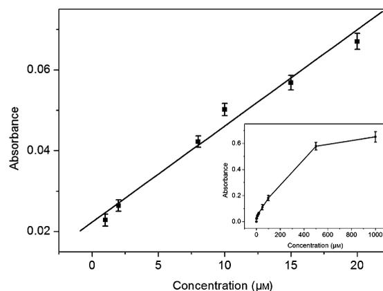
**Figure 3.** The linear calibration plot of the absorbance at 651 nm on the concentration of H<sub>2</sub>O<sub>2</sub> from 1 to 20 μM. The inset shows dependence of the absorbance at 651 nm on the concentration of H<sub>2</sub>O<sub>2</sub> in the range from 0 to 1 mM.
