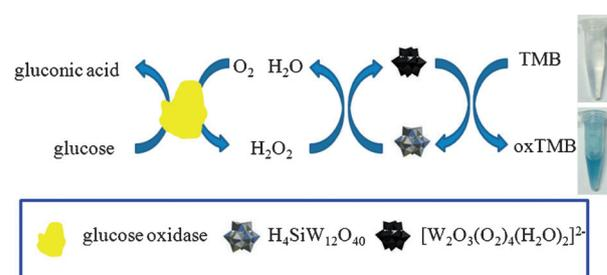
**Figure 5.** An illustration (not to scale) of the colorimetric detection of  $\text{H}_2\text{O}_2$  and glucose using HSiW as a peroxidase-like catalyst.
