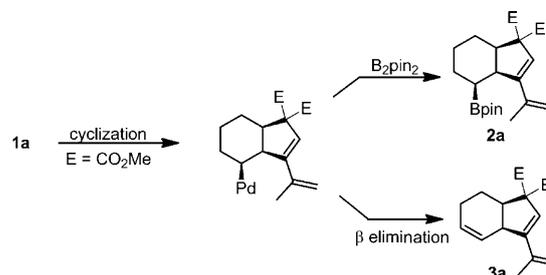
**Scheme 2.** Cleavage of the Pd–C bond by a boron-containing reagent vs.  $\beta$  elimination.
