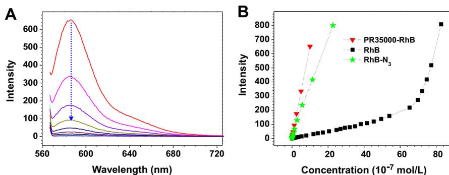
Fig. 4. (A) Fluorescence emission spectra of RhB-PR1C in DMSO solution with gradient concentrations from 0.05 mg/mL to  $9.8 \times 10^{-5}$  mg/mL (along the arrow) by step-wise dilution. (B) Fluorophores concentration versus fluorescence emission intensity of RhB, RhB- $N_3$ , RhB-PR1C in DMSO solution. All the fluorescence emission spectra were excited at 564 nm and the emission peak points were at 587 nm. The emission slit was 3 nm.
