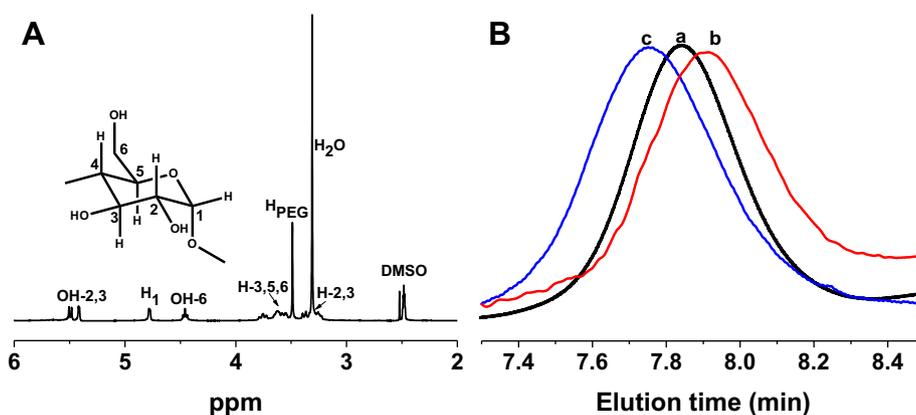
Fig. 2. (A)  $^1\text{H}$  NMR spectrum of the polyrotaxane prepared from PEG 35 kDa, mono-alkyne quaternary ammonium salt and  $\alpha$ -CD in DMSO. (B) Typical GPC curves of (a) PR1A-VC, (b) PR1B-VC, and (c) PR1C-VC.
