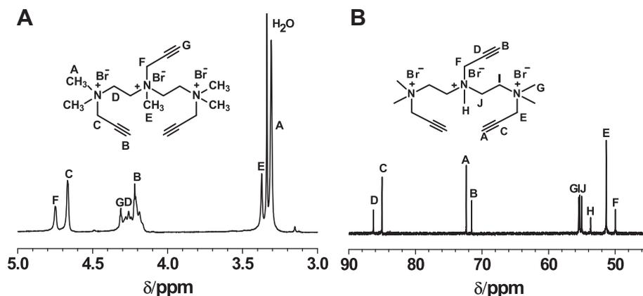
Fig. 1. (A)  $^1\text{H}$  NMR spectrum of tri-alkyne quaternary ammonium salt in  $\text{DMSO}-d_6$ , (B)  $^{13}\text{C}$  NMR spectrum of tri-alkyne quaternary ammonium salt in  $\text{DMSO}-d_6$ .
