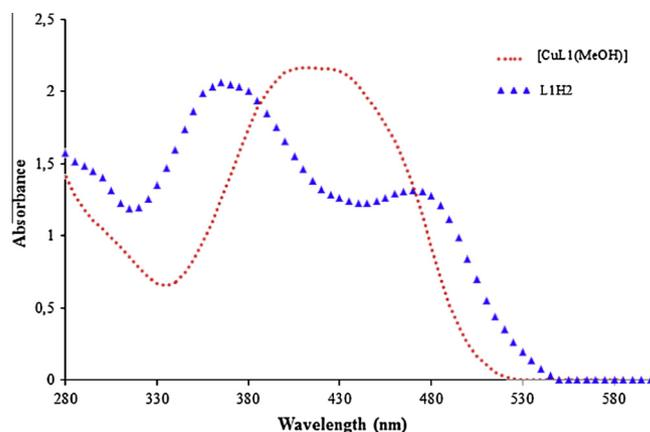
Fig. 10. UV-Vis. spectra of the ligand  $\text{L}^1\text{H}_2$  and its Cu(II) complex in DMF.
