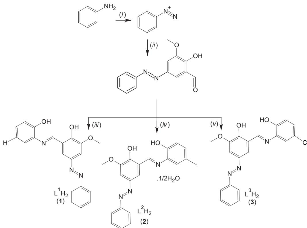
**Scheme 1.** The general preparation route of azo-azomethines. (i)  $\text{NaNO}_2$ ,  $\text{HCl}$ ,  $0^\circ\text{C}$ , (ii) 2-hydroxy-3-methoxybenzaldehyde, (iii) 2-aminophenol, (iv) 2-amino-*p*-cresol, and (v) 2-amino-4-chlorophenol.
