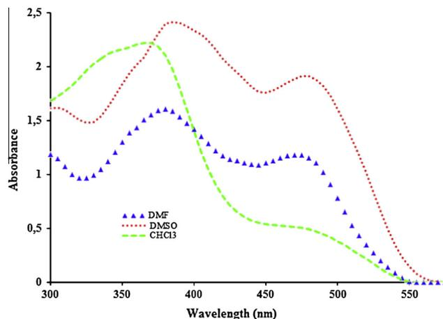
Fig. 7. UV-Vis. spectra of  $\text{L}^2\text{H}_2 \cdot 1/2\text{H}_2\text{O}$  ligand in solvents DMSO, DMF and  $\text{CHCl}_3$ .
