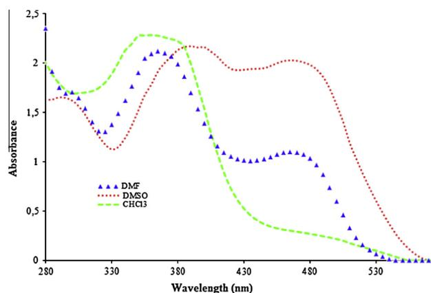
Fig. 8. UV-Vis. spectra of  $\text{L}^3\text{H}_2$  ligand in various solvents.
