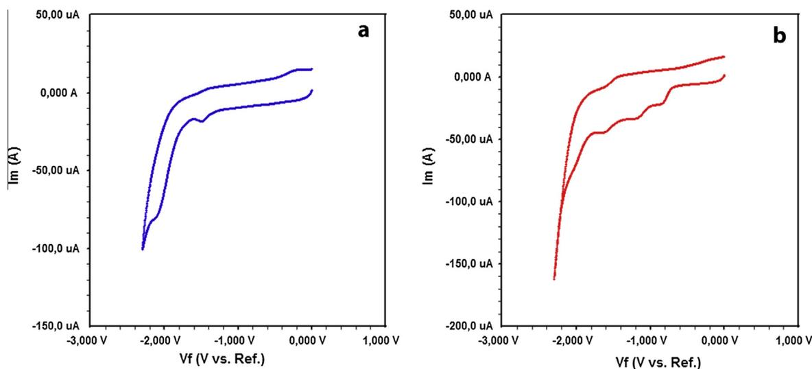
**Fig. 11.** Cyclic voltammograms recorded for the reduction of 1.0 mM  $L^1H_2$  (a) and  $[CuL^1(MeOH)]$  (b) at a GC electrode in DMSO containing 0.1 M TBATFB in the range from 0 to  $-2.3$  V. Scan rate is  $100\text{ mV s}^{-1}$ .
