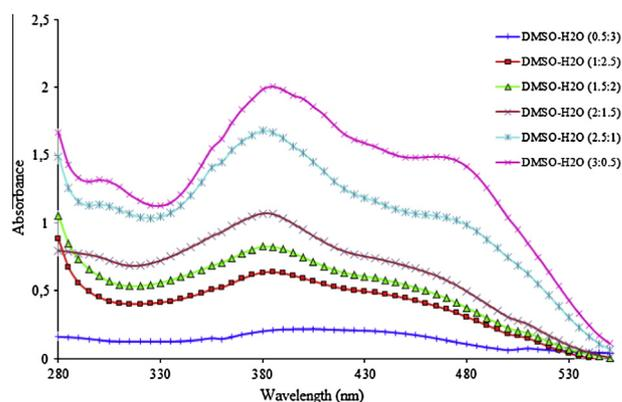
Fig. 9. UV-Vis. spectra of  $\text{L}^2\text{H}_2\cdot 1/2\text{H}_2\text{O}$  ligand in DMSO- $\text{H}_2\text{O}$  mixtures.
