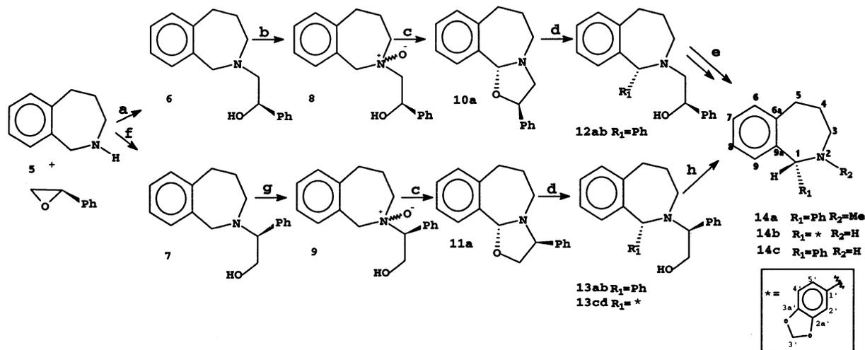
**Scheme 1.** Reagents and conditions: (a) NaH, THF, 80°C; (b) H<sub>2</sub>O<sub>2</sub> 30%, MeOH, 10°C; (c) BuLi, THF, -78°C; (d) RMgBr, THF, -78°C; (e) MeI, CH<sub>3</sub>CN, 60°C, *t*-BuOK/*t*-BuOH, 80°C; (f) CH<sub>3</sub>CN, LiClO<sub>4</sub>, 30°C; (g) H<sub>2</sub>O<sub>2</sub> 30%, MeOH, rt; (h) H<sub>2</sub> Pd/C.
