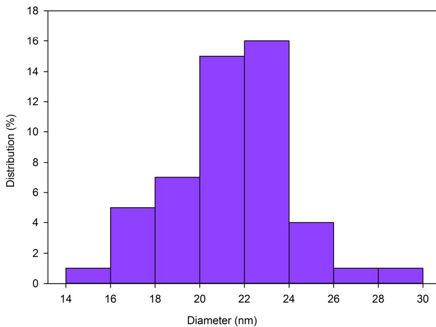
**Fig. 8.** Particle size distribution of catalyst
