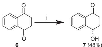
Scheme 2. Biotransformation of 1,4-naphthoquinone (**6**). (i) *P. variabile* resting cells, 8 h, phosphate buffer, 25 °C.
