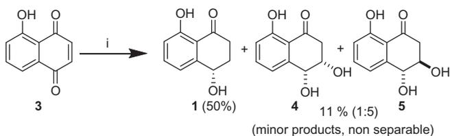
**Scheme 1.** Biotransformation of juglone (**3**). (i) *P. variabile* resting cells, 48 h, phosphate buffer, 25 °C.
