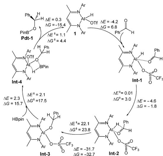
**Scheme 2.** Reaction mechanism for the hydroboration of benzaldehyde calculated at the M06/def2-TZVPP/BP86/def2-SVP level of theory.<sup>[11b]</sup>
