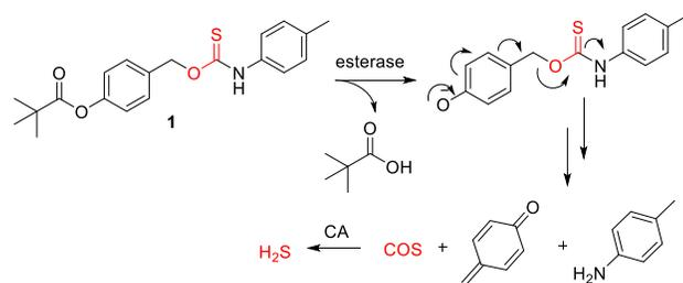
**Scheme 1.** Design of esterase-triggered self-immolative COS/H<sub>2</sub>S donors and proposed COS/H<sub>2</sub>S release mechanism.
