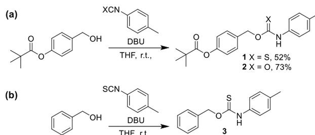
**Scheme 2.** (a) Synthesis of H<sub>2</sub>S donor **1**, CO<sub>2</sub>-releasing analogue **2**, and triggerless thiocarbamate **3**.
