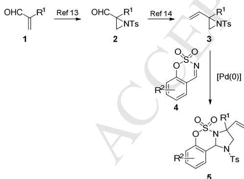
**Scheme 3.** Straightforward access to 2-substituted vinylaziridines **3** and reaction with cyclic *N*-sulfonyl imines **4**.
