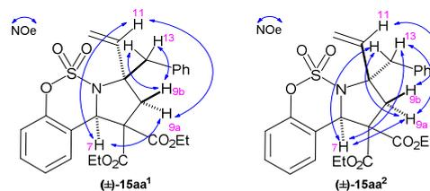
Scheme 11. Relative configuration of ( $\pm$ )-**15aa**<sup>1</sup> and ( $\pm$ )-**15aa**<sup>2</sup> via NOESY experiments.<sup>25</sup>
