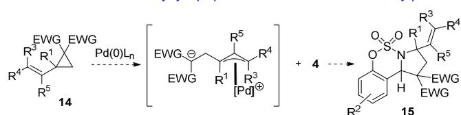
**Scheme 6.** New targeted objectives within the Pd-catalyzed (3+2)-cycloaddition reactions with 2-substituted vinyl-aziridines and cyclopropanes.
