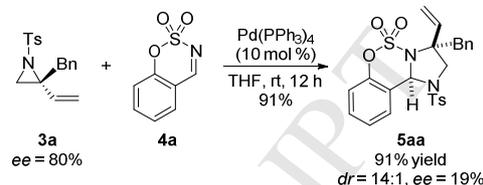
**Scheme 7.** Prior trial on an asymmetric version from enantioenriched 2-substituted vinylaziridine **3a** (80% *ee*).
