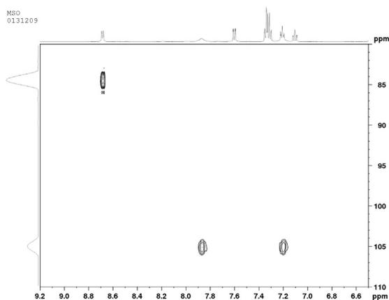
**Fig. 3.**  $^1\text{H}$ – $^{15}\text{N}$  correlation spectrum of compound **2** (HSQC) in  $\text{DMSO}-d_6$  solution at 298 K. The horizontal axis shows 1D  $^1\text{H}$  spectrum; the vertical axis shows  $^{15}\text{N}$  projection.
