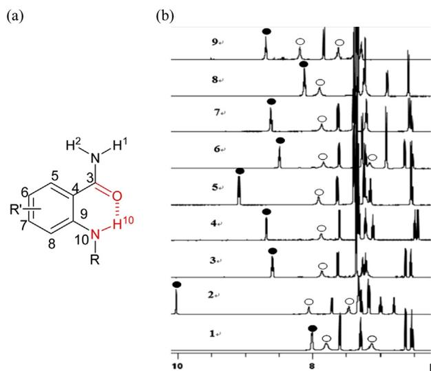
Fig. 1. (a) Structures with intramolecular hydrogen bonds. (b) Partial picture of <sup>1</sup>H NMR spectra of compounds **1–9** in DMSO-*d*<sub>6</sub> solution at 298 K, H-10: solid circle, H-1 and H-2: hollow circle.
