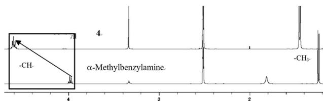
Fig. 6. Partial picture of  $^1\text{H}$  NMR spectra of compound **4** and  $\alpha$ -methylbenzylamine in  $\text{DMSO-}d_6$  solution at 298 K.
