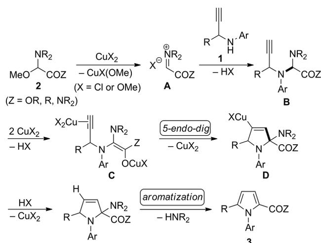
Scheme 3. A plausible reaction mechanism for copper-catalyzed [4+1] annulation.
