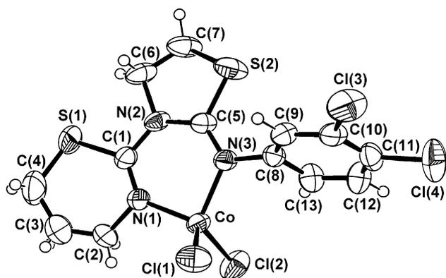
Fig. 2. Molecular structure of  $[\text{CoCl}_2(\text{TdTz})]$  (**2**), showing the atom numbering scheme. The thermal ellipsoids are drawn at the 50% level.
