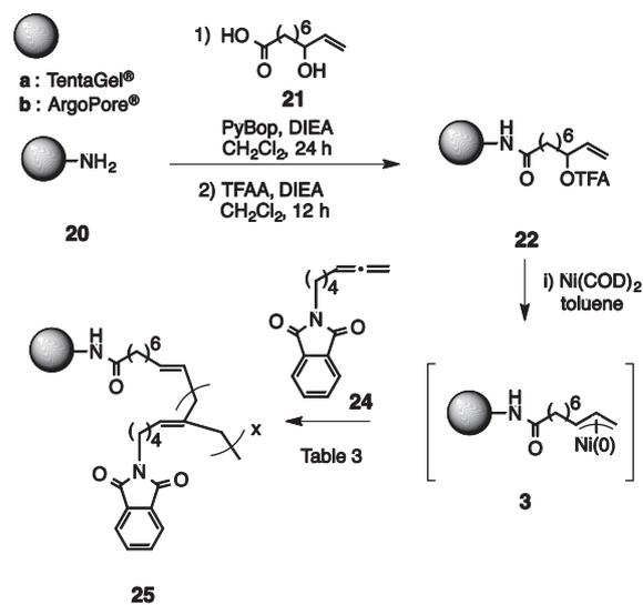
Scheme 4. Synthesis of the solid-supported polymer 25.
