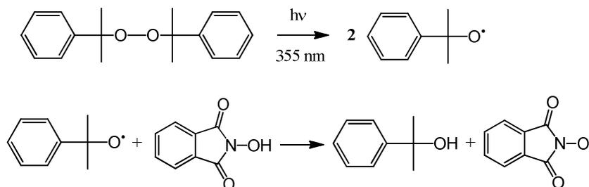
**Scheme 2.** Generation of PINO by laser flash photolysis
