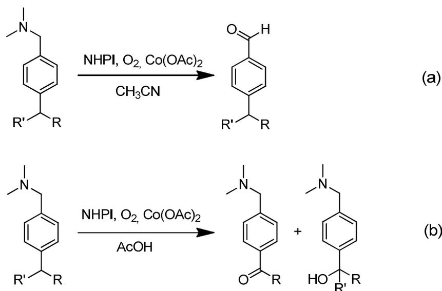
**Figure 3.** Products formed in the aerobic oxidation of 4-X-N,N-dimethylbenzylamines **1-3** catalyzed by NHPI (a) in CH<sub>3</sub>CN and (b) in AcOH.
