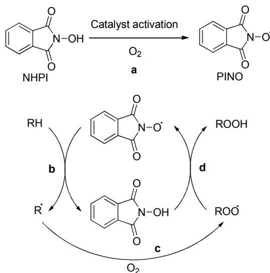
21 **Scheme 1.** Catalytic cycle for the aerobic oxidation of hydrocarbons catalyzed by NHPI
