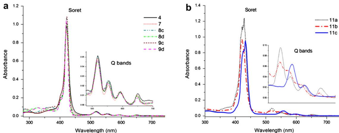
**Fig. 1.** (a) Electronic absorption spectra of porphyrins **4**, **7**, **8c**, **8d**, **9c** and **9d** in  $\text{CHCl}_3$  at 298 K. (b) Electronic absorption spectra of  $\beta$ ,*meso*-benzoxazolyl-bridged porphyrin dyads (**11a–c**) in  $\text{CHCl}_3$  at 298 K. Inset in both (a) and (b) shows the Q bands.
