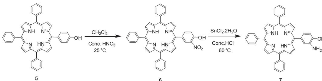
Scheme 2. Synthesis of 5-(3-amino-4-hydroxyphenyl)-10,15,20-triphenylporphyrin.
