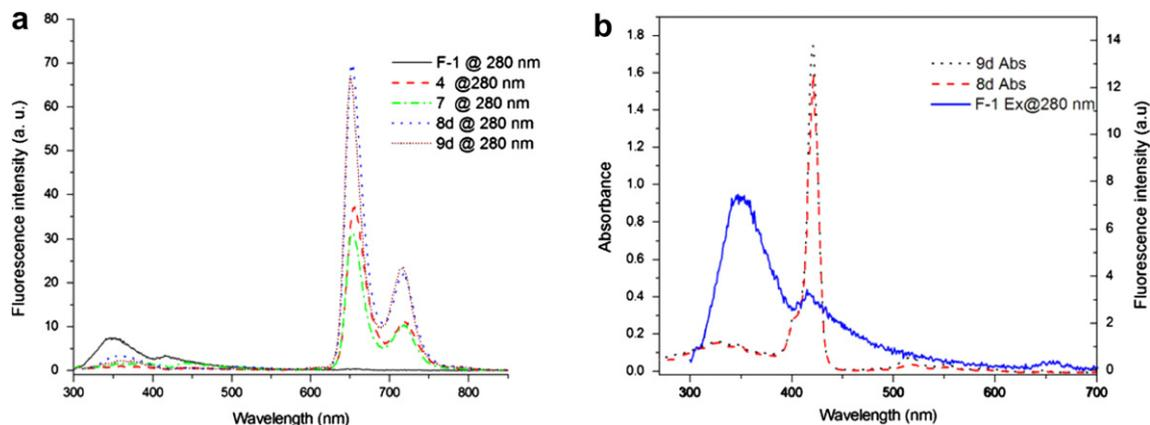
**Fig. 4.** (a) Fluorescence spectra of **F-1** and porphyrins **4**, **7**, **8d** and **9d** in  $\text{CHCl}_3$  ( $2 \times 10^{-6} \text{ mol L}^{-1}$ ) at 298 K,  $\lambda_{\text{ex}} = 280 \text{ nm}$  (b) UV-Vis spectra of **8d** and **9d** and fluorescence spectrum of **F-1** ( $\lambda_{\text{ex}} = 280 \text{ nm}$ ) in  $\text{CHCl}_3$ .
