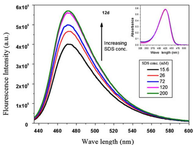
**Fig. 10** Emission and absorption spectra (inset) of **12d** in PBS with different SDS conc
