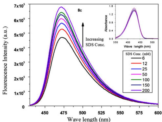
**Fig. 9** Emission and absorption spectra (inset) of **8c** in PBS with different SDS conc
