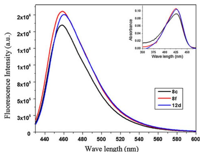
**Fig. 6** Emission and absorption spectra (inset) of **8c**, **8f**, **12d** in DCM
