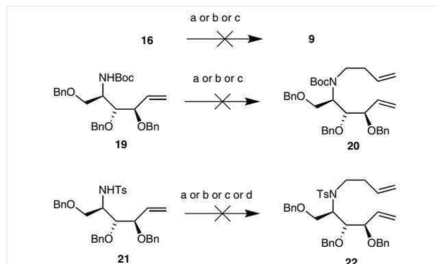
**Scheme 5** Reagents and conditions: (a) 4-bromobut-1-ene,  $\text{K}_2\text{CO}_3$ , DMF,  $0^\circ\text{C}$  to r.t.; (b) 4-bromobut-1-ene,  $\text{Et}_3\text{N}$ ,  $\text{CH}_2\text{Cl}_2$ ,  $0^\circ\text{C}$  to r.t.; (c) 4-bromobut-1-ene,  $\text{NaH}$ , THF, TBAI,  $60^\circ\text{C}$ ; (d)  $\text{PPh}_3$ , DIAD, phthalimide, 1-butanol, THF.
