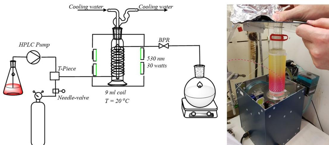
**Figure 1.** Schematic overview and picture of the photochemical reactor with green LED chips.
