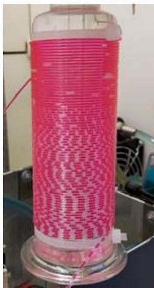
**Figure 2.** Oxygen consumption seen over the length of the coil at a 3 mL/min flow rate.
