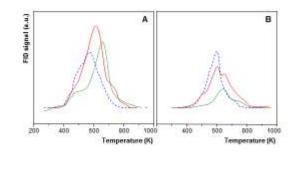
**Figure 6:** Temperature programmed oxidation (TPO) profiles for the catalyst tested at the same reaction conditions  $W/F_{furfural} = 3 g_{cat}.h.(g_{furfural})^{-1}$ ;  $W/F_{total} = 0.023 g_{cat}.h.(g_{feed})^{-1}$ ;  $H_2/Furfural molar ratio = 245$ ; T=573 K. (I) Fe<sub>15</sub>; (II) Fe<sub>7</sub>Pt<sub>0.07</sub>; (III) Fe<sub>5</sub>Pt<sub>0.5</sub>; and (IV) Pt<sub>1.7</sub>.
