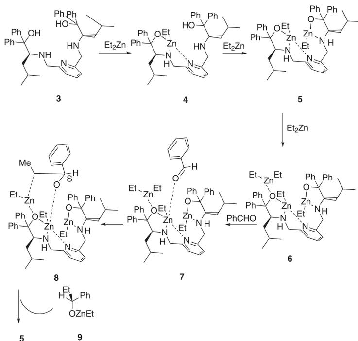
Figure 2. The proposed catalytic mechanism.
