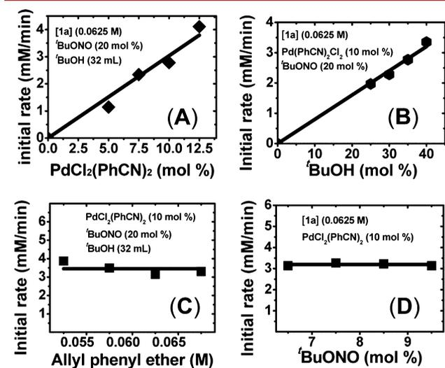
**Figure 1.** Dependence of the initial rate on (A) [Pd(PhCN)<sub>2</sub>Cl<sub>2</sub>] (first-order); (B) [tBuOH] (first-order); (C) [1a] (zeroth-order); (D) [tBuONO] (zeroth-order). Conditions: 1a, Pd(PhCN)<sub>2</sub>Cl<sub>2</sub> (5–12.5 mol %), tBuONO (20 mol % for A–C, 6.5–9.5 mol % for D), tBuOH, O<sub>2</sub> (1 atm). For details, see [Supporting Information](#).
