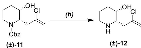
*Synthesis of 12.* A 50 L glass reactor was charged with crude **11** (3.50 kg), HCl<sub>(aq)</sub> (6 M, 18.83 L) and EtOH (20 L). The reaction mixture was refluxed for about 30 h. After completion of the reaction, the mixture was concentrated under reduced pressure at 50–55 °C to remove EtOH. To the residual liquid was added with MTBE (2 × 20 L), and resulting mixture was stirred for a few
