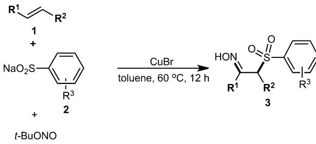
**Scheme 1.** Difunctionalization reaction of alkenes via the incorporation of the sulfonyl group.
