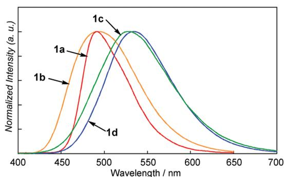
**Figure 1.** Chemiluminescence spectra of dioxetanes **1a–d**.
