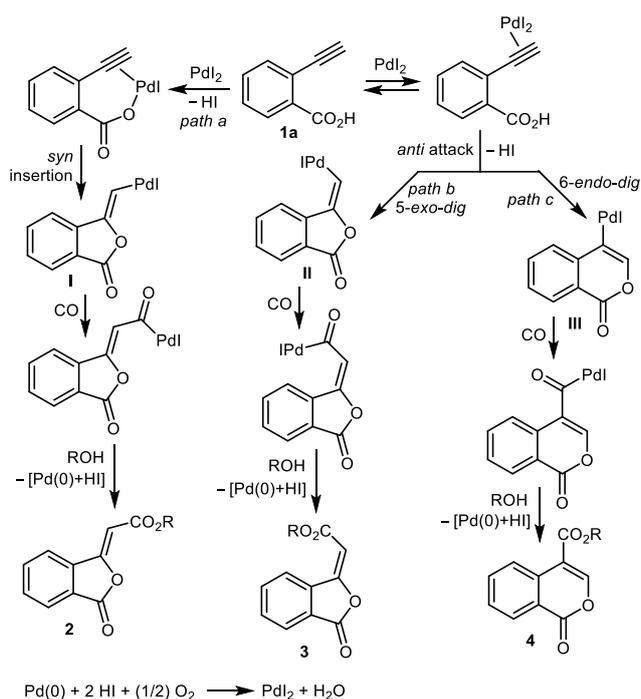
**Scheme 1.** Possible divergent pathways in the PdI<sub>2</sub>-catalyzed oxidative cyclization-alkoxycarbonylation of 2-ethynylbenzoic acid **1a**.
