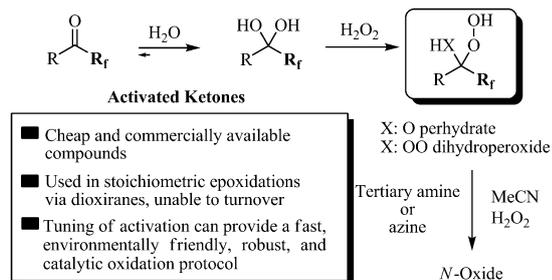
Scheme 1. Design of the synthesis of *N*-oxides.
