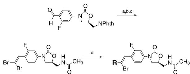
**Scheme 2.** Synthesis of bromostilbenes: (a) polystyrene-PPh<sub>3</sub> (6 equiv), CBr<sub>4</sub> (3 equiv), CH<sub>2</sub>Cl<sub>2</sub>, -5 °C, 1 h, 93%; (b) N<sub>2</sub>H<sub>4</sub>-H<sub>2</sub>O (3 equiv), THF/EtOH, 70 °C, 3 h; (c) Ac<sub>2</sub>O, pyridine, rt, 5 min, 77% total for (b) + (c); (d) R-B(OH)<sub>2</sub>, Pd(PPh<sub>3</sub>)<sub>4</sub> (0.1 equiv), 10% Na<sub>2</sub>CO<sub>3</sub>/H<sub>2</sub>O, DME, 70 °C, 16 h.
