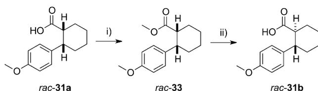
Scheme 11. Reaction conditions: i) MeOH, H<sub>2</sub>SO<sub>4</sub> (catalytic), reflux, 5 h; ii) NaOMe, MeOH, 80 °C, 4 h then HCl (1 M).
