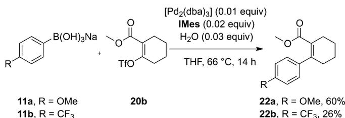
Scheme 6. Optimized reaction conditions for the Suzuki-Miyaura cross-coupling by using trifluoromethanesulfonate **20b**.
