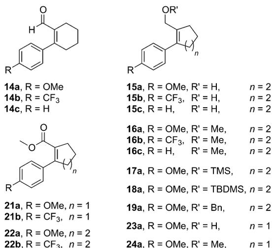
Scheme 7. Substrates applied in the Ir-catalyzed asymmetric hydrogenation reaction (TMS = trimethyl silyl; TBDMS = *tert*-butyl dimethyl silyl; Bn = benzyl).
