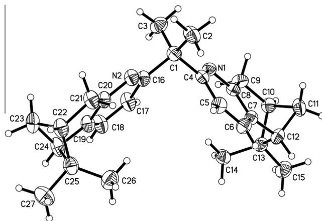
**Figure 1.** X-ray crystal structure of 2,2-dipyridylpropane **9** (hexagonal crystal system and P6(1) space group; CCDC number: 963556).
