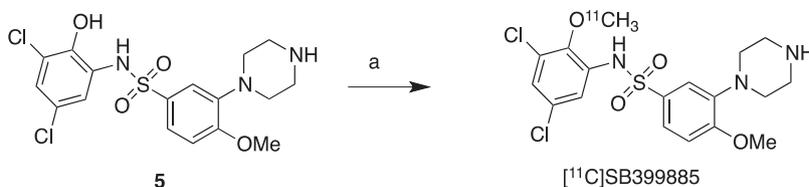
**Scheme 2.** Radiosynthesis of  $[^{11}\text{C}]\text{SB399885}$ . Reagents and conditions: (a)  $[^{11}\text{C}]\text{CH}_3\text{OTf}$ , NaOH, acetone, rt, 5 min.
