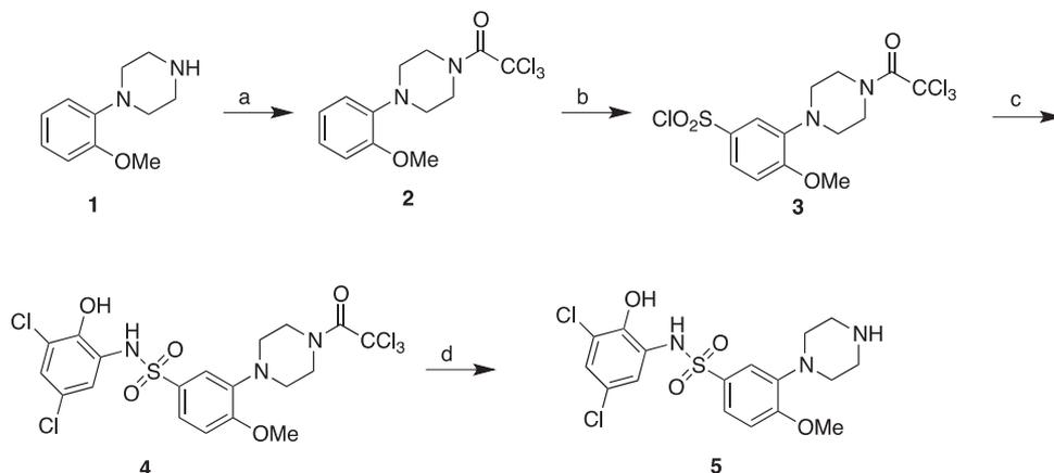
**Scheme 1.** Synthesis of **5**. Reagents and conditions: (a) CCl<sub>3</sub>COCl, CH<sub>2</sub>Cl<sub>2</sub>, rt, 4 h: 87%; (b) ClSO<sub>2</sub>OH, CH<sub>2</sub>Cl<sub>2</sub>, rt, 1 h: 77.5%; (c) 2-amino-4,6-dichlorophenol, CH<sub>2</sub>Cl<sub>2</sub>, pyridine, 0 °C, overnight: 96%; (d) KOH, THF, reflux, 20 h, 74%.
