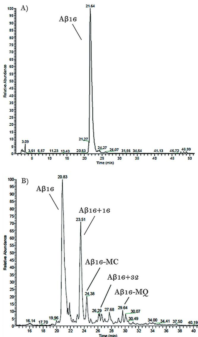
**Figure 4.** HPLC-MS elution profiles of A $\beta$ 16 (75  $\mu$ M) in HEPES buffer (50 mM) pH 7.4 at 25  $^{\circ}$ C, in the presence of copper(II) (25  $\mu$ M) and MC (3 mM) at the beginning (A), and after 90 min incubation time (B). The assignment of the peaks is shown.
