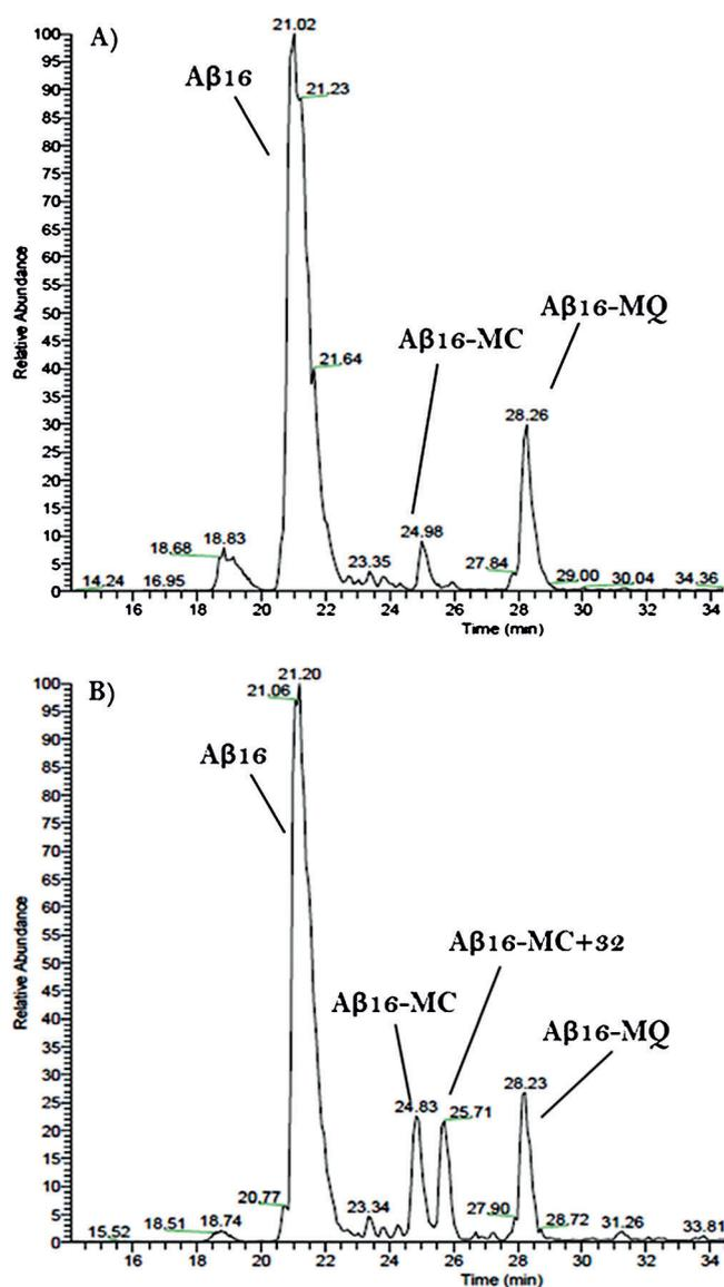
**Figure 5.** HPLC-MS elution profiles of A $\beta$ 16 (75  $\mu$ M) in HEPES buffer (50 mM) pH 7.4 at 25  $^{\circ}$ C in the presence of MC after A) 90 min and B) 450 min reaction time. The assignment of the peaks is shown.
