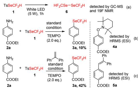
**SCHEME 5.** Investigations to elucidate the reaction mechanism
