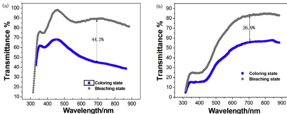
**Fig. 5.** The optical contrast of the electroactive materials at the coloring and bleaching state in ACN solution containing 0.05 M TBAP and 0.05 M LiClO<sub>4</sub>. a: WO<sub>3</sub> film and b: WO<sub>3</sub>/P3TPA film.
