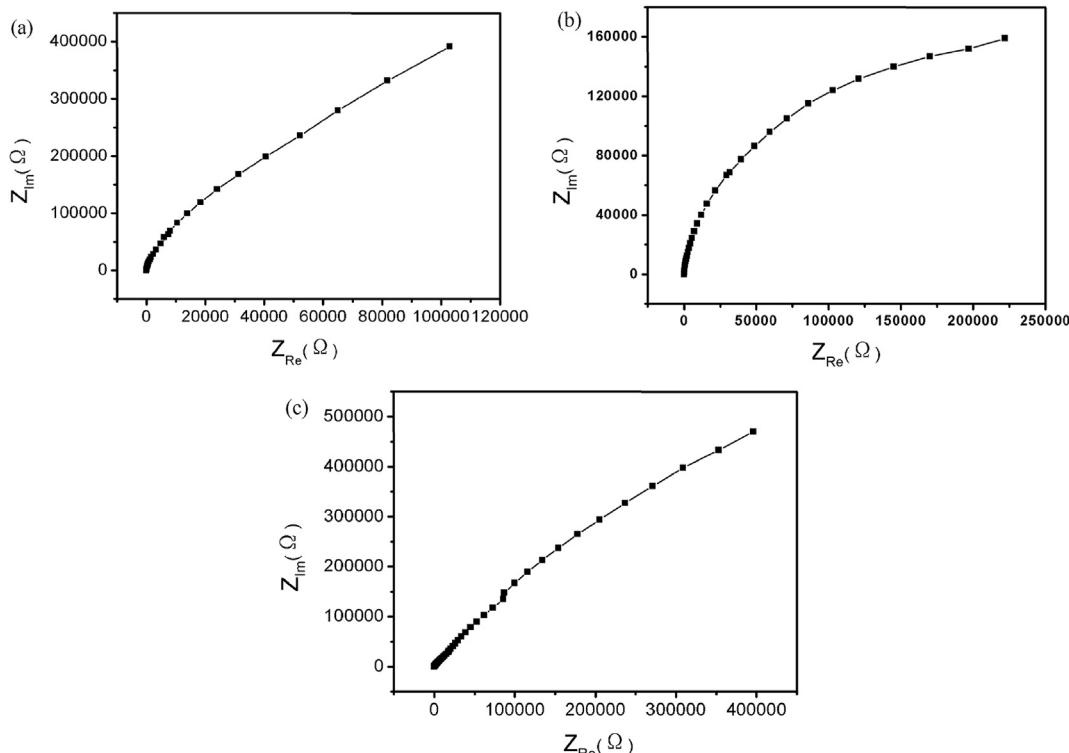
**Fig. 8.** The AC impedance diagrams of (a)  $\text{WO}_3$  film, (b) P3TPA film, (c)  $\text{WO}_3/\text{P3TPA}$  film.
