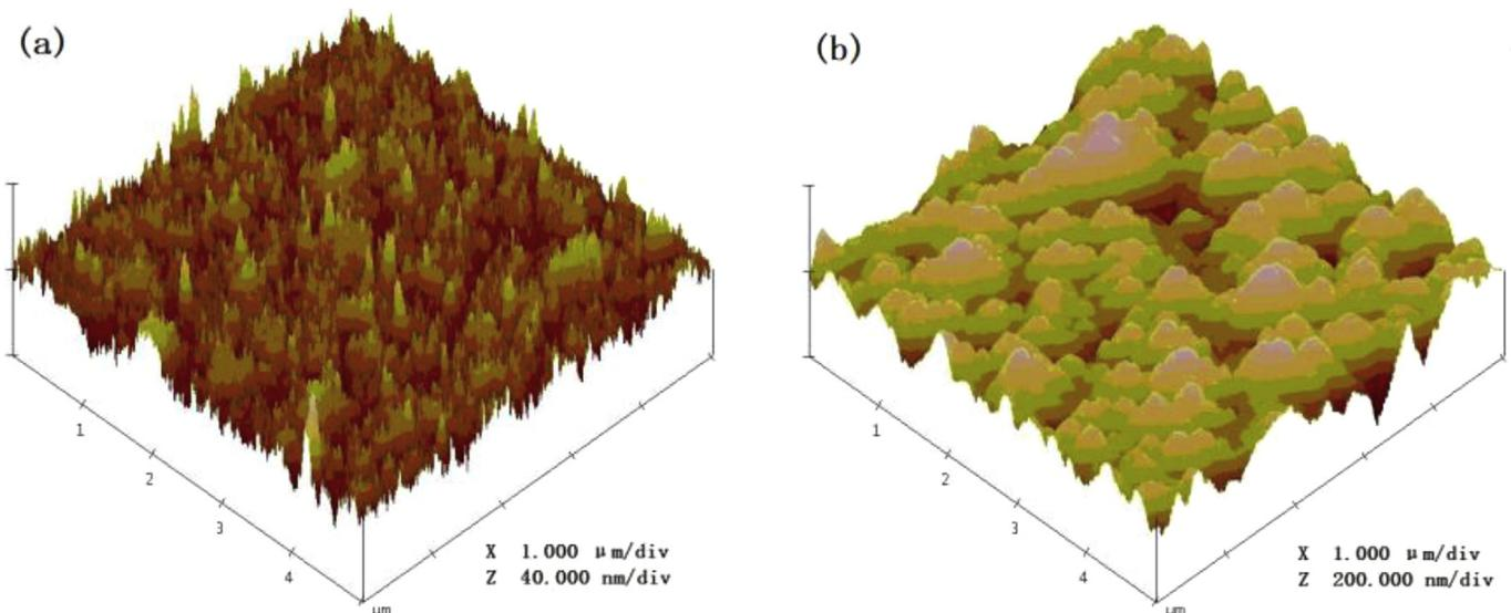
**Fig. 3.** The AFM images of the (a)  $\text{WO}_3$  film and (b)  $\text{WO}_3/\text{P3TPA}$  film.
