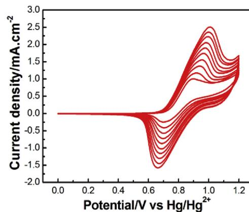
**Fig. 1.** The electropolymerization of 3TPA ( $5.0 \times 10^{-2}$  M) at 100 mV/s for ten times in the ACN solution with 0.1 M TBAP.
