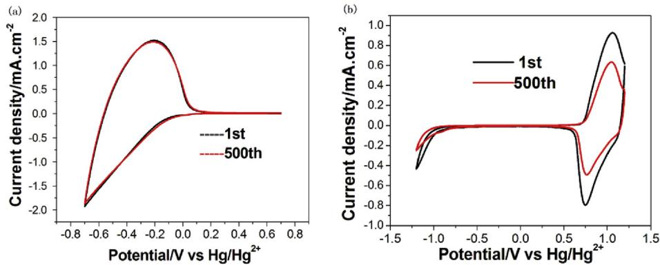
**Fig. 7.** The CV of active materials for the 1st and 500<sup>th</sup> cycle in the ACN solution containing 0.05 M TBAP-0.5 M LiClO<sub>4</sub>. Scan rate = 100 mV/s. a:  $\text{WO}_3$  film and b:  $\text{WO}_3/\text{P3TPA}$  film.
