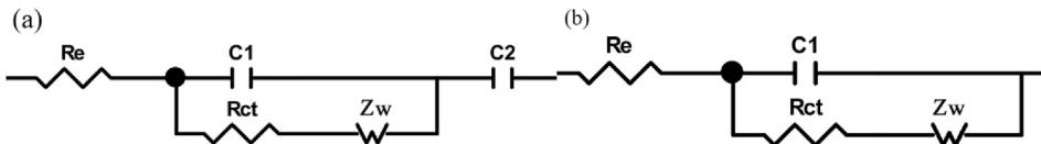
**Fig. 9.** The equivalent circuit used for fitting the experimental impedance data (a)  $\text{WO}_3$  film, (b) P3TPA film and  $\text{WO}_3/\text{P3TPA}$  film.
