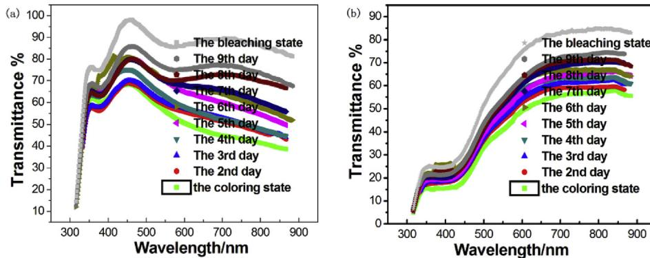
**Fig. 4.** The open-circuit memory of electroactive materials in the ACN solution containing 0.05 M TBAP and 0.05 M LiClO<sub>4</sub>. a: WO<sub>3</sub> film and b: WO<sub>3</sub>/P3TPA film.
