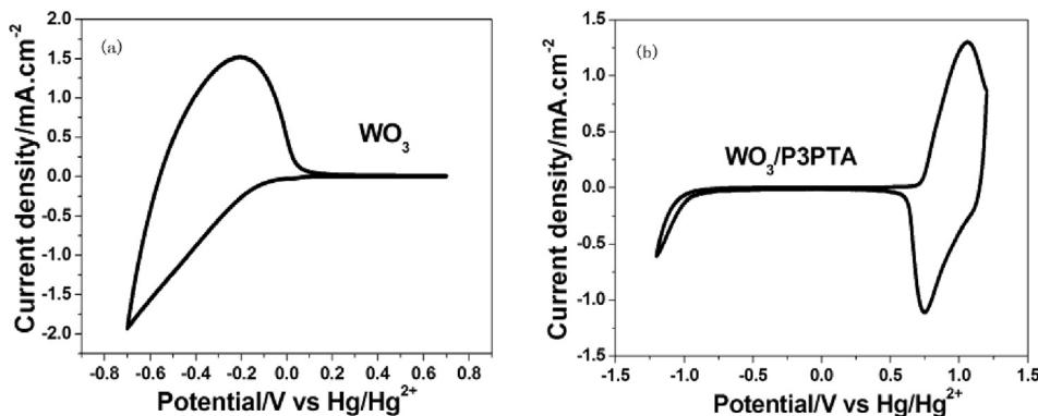
**Fig. 6.** The CV of the electroactive materials in the CAN solution containing 0.05 M TBAP–0.05 M LiClO<sub>4</sub>. Scan rate = 100 mV/s. a: WO<sub>3</sub> film; b: WO<sub>3</sub>/P3TPA film.
