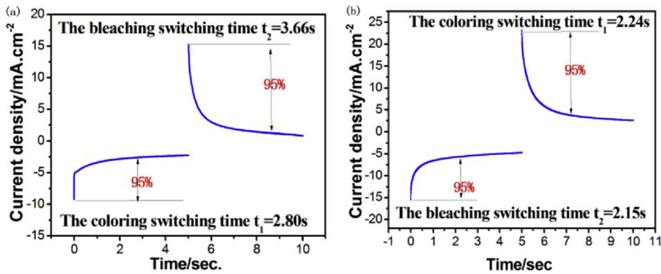
**Fig. 2.** The coloring time and bleaching time of the electroactive film in the ACN solution with 0.05 M TBAP and 0.05 M LiClO<sub>4</sub>. a:  $\text{WO}_3$  film and b:  $\text{WO}_3/\text{P3TPA}$  film.
