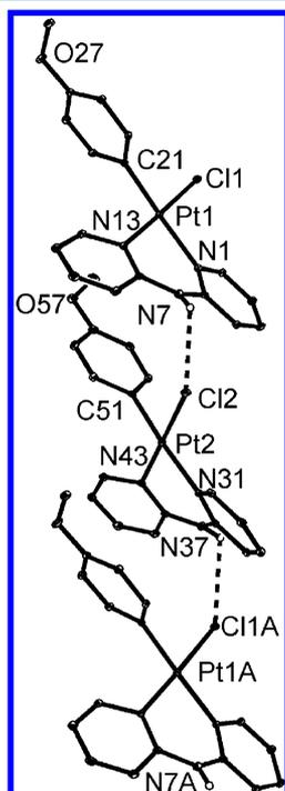
**Figure 5.** Supramolecular polymer formed by NH...Cl hydrogen bonding in **6b**. H-bonding distances (Å): N(7)...Cl(2) 3.384(4); N(37)...Cl(1) 3.351(4).
