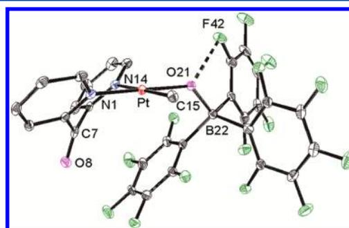
Figure 1. View of the structure of complex **2a**. Selected bond parameters (distances in Å, angles in deg): Pt-N(1) 1.975(5); Pt-N(14) 2.122(5); Pt-C(15) 2.044(7); Pt-O(21) 2.047(4); N(1)-Pt-N(14) 88.5(2).
