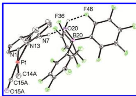
**Figure 2.** View of the structure of complex **3b**. Selected bond parameters (distances in Å; angles in deg): Pt–N(1) 2.110(6); Pt–N(13) 2.083(6); Pt–C(14A) 2.08(2); Pt–C(15A) 1.82(1); C(15A)–O(15A) 1.14(1); N(1)PtN(13) 87.2(2).
