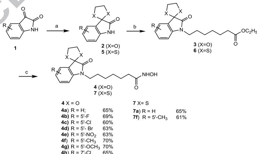
Scheme 1. Synthesis of 2'-oxospiro[1,3]dioxolane/dithiolane-2,3'-indoline-based hydroxamic acids. Reagents and conditions: a) ethylene glycol/ethylene dithiol, *p*-TsOH, toluene, Δ, 24 h; b) ethyl 7-bromoheptanoate, K<sub>2</sub>CO<sub>3</sub>, KI, DMF, 60 °C, 24 h; c) hydroxylamine hydrochloride, NaOH, MeOH/THF, -5 °C, 30-60 min.
