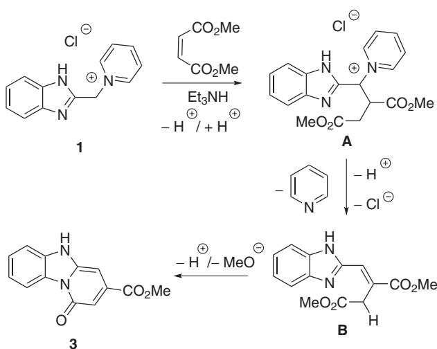
**Scheme 4:** Proposed mechanism for the formation of **3**.
