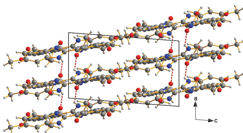
**Fig. 2:** View of the crystal structure of **2a** in a projection along [010] showing the formation of layers parallel to the (301) plane of **2a**. Hydrogen bonds are shown as red dashed lines (N–H…O) connecting these layers.
