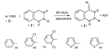
The reaction also took slowly place at room temperature, but the reaction was generally incomplete after 24h. The condensation products was obtained in good yields under focused microwave irradiation (2450 MHz, 60 W, 6 min.) with a resonance cavity  $^4$  the results are reported in table I.
