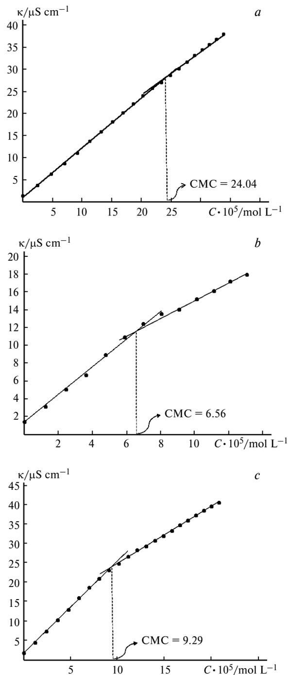
**Fig. 2.** Conductivity as a function of surfactant concentration for the determination of critical micelle concentration of compounds **4a** (a), **4b** (b), and **5b** (c).
