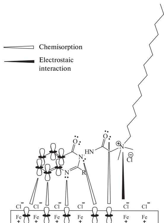
**Fig. 3.** The possible corrosion inhibition mechanism for the cationic surfactants.
