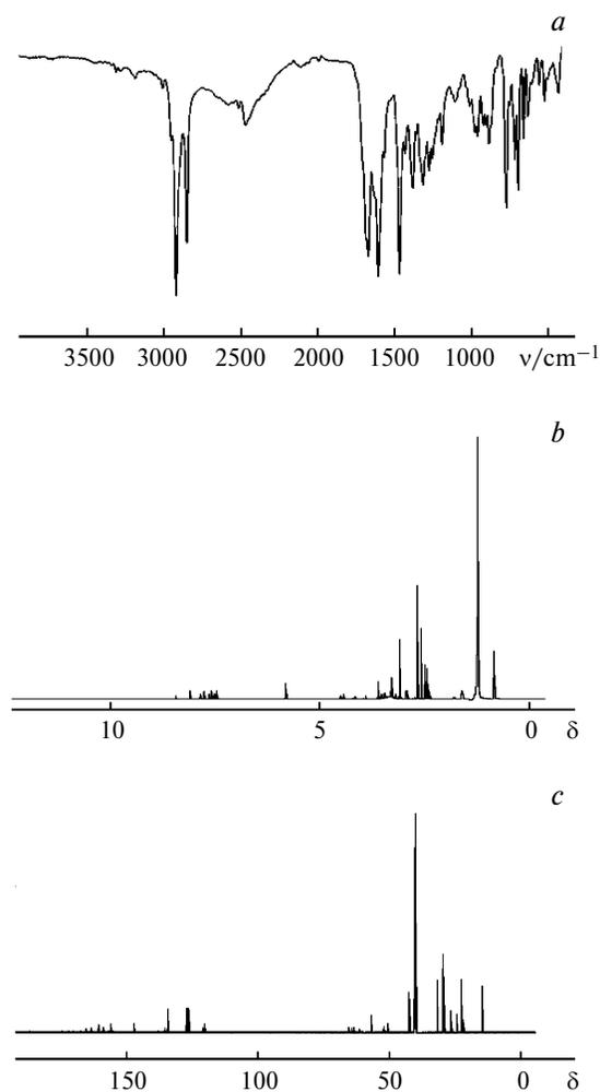
**Fig. 1.** The FT-IR (a),  $^1\text{H}$  (b) and  $^{13}\text{C}$  NMR (c) spectra of compound **4a**.
